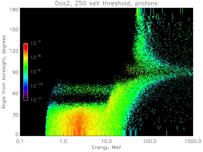
The higher threshold of Dos2 increases the energy at which response turns on (lower left), and also suppresses response to high-energy, low-dE/dx protons (right) as for the 1-MeV threshold on Dos3. I have supplied full position and direction information from these simulations to Paul O'Brien, as I have done for MagEIS and RPS simulations, so he can assemble response libraries as needed.
