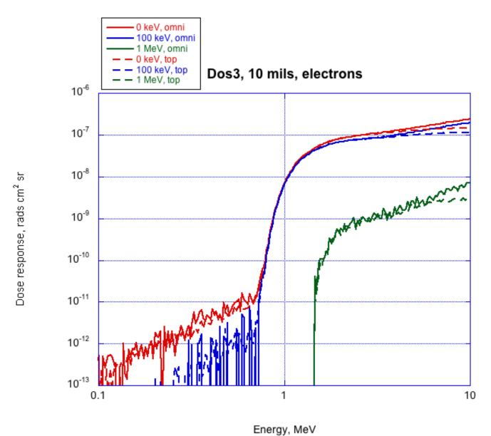
Here is the response of Dos3 without the thinned window. Here and in other Dos3 plots, I show the response with no threshold (all dose counted), and with a threshold of 100 keV or 1 MeV per event. The value plotted is the response in dose per unit fluence; multiply by fluence in particles per (cm² sr) to get dose in rads (or integrate over energy for a spectrum), or by flux in particles per (cm² sr s) to get dose rate in rads per second.
