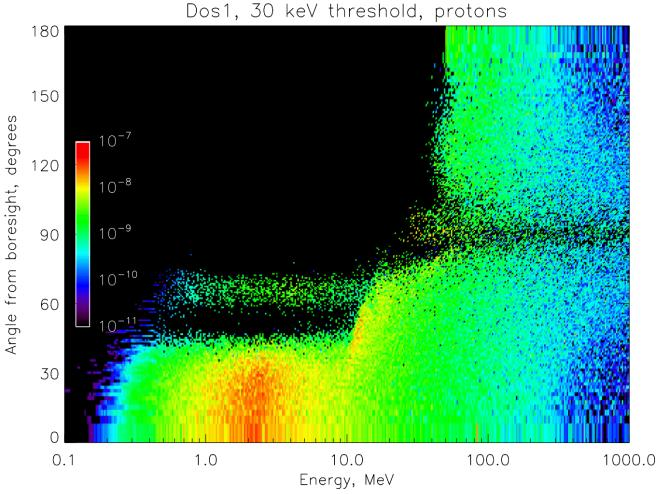
Protons scatter less in the 1.8- $\mu$ m foil, so a spike due to the response through the second aperture around 60° off axis is easier to see in this plot for Dos1. As seen on slide 11, with its low threshold it accounts for essentially all proton dose; the falloff at right is not due to suppression of events, but simply to declining dE/dx.
