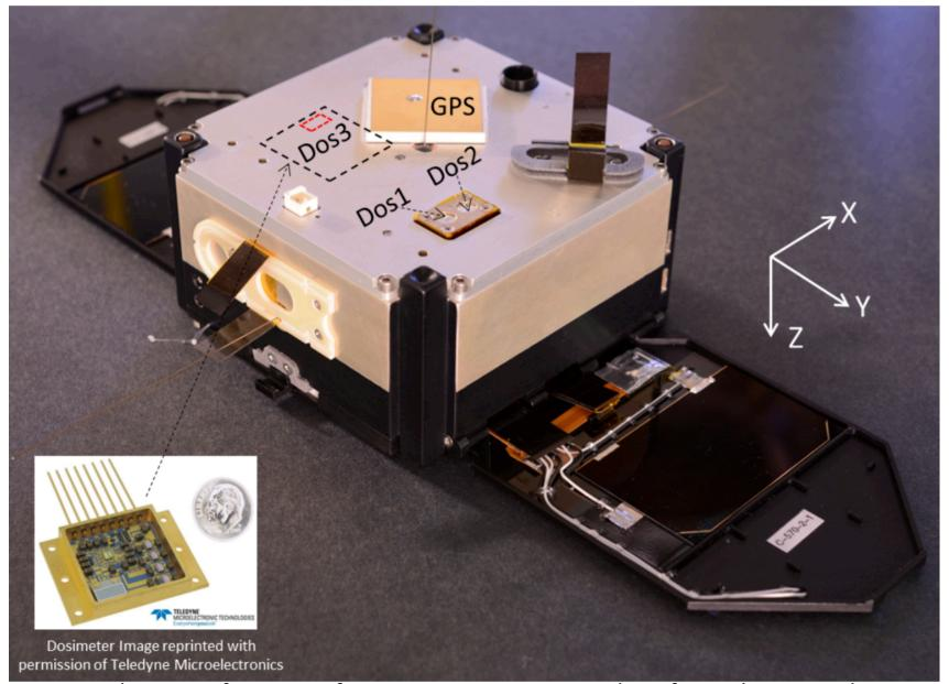
This is a reproduction of Figure 3 from TOR-2016-01155, identifying the microdosimeters. Dos1 and Dos2 are silicon detectors 1.8 mm in diameter and 60  $\mu$  thick, shielded by 1.8  $\mu$  of aluminum foil; Dos3 is a silicon chip 3 mm x 7 mm x 250  $\mu$  under a 10-mil Kovar lid, possibly thinned to 4 mils over the chip, and an Al top panel thinned to 20 mils above the package.
