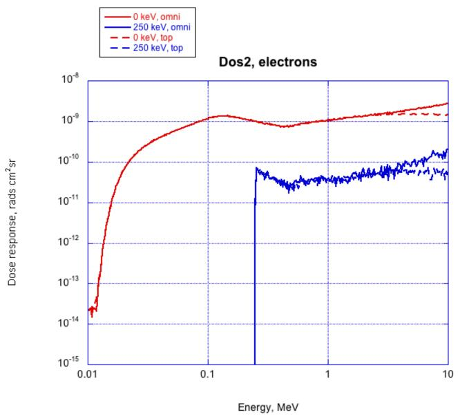
Here is the response of Dos2 to electrons. The higher threshold, like the 1-MeV threshold in the Teledyne microdosimeter (slides 5 and 6) suppresses response to most electron particle events.
