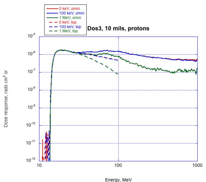
Here is the Dos3 response to protons without the thinned window. In all these plots, the dashed lines indicate the results of simulations with particles incident only in a circle right above the microdosimeter; each dashed line diverges from its solid line where we start to see response to penetration through the spacecraft away from each microdosimeter. Later in this report, I present plots of response vs. angle, which makes this more clear.
