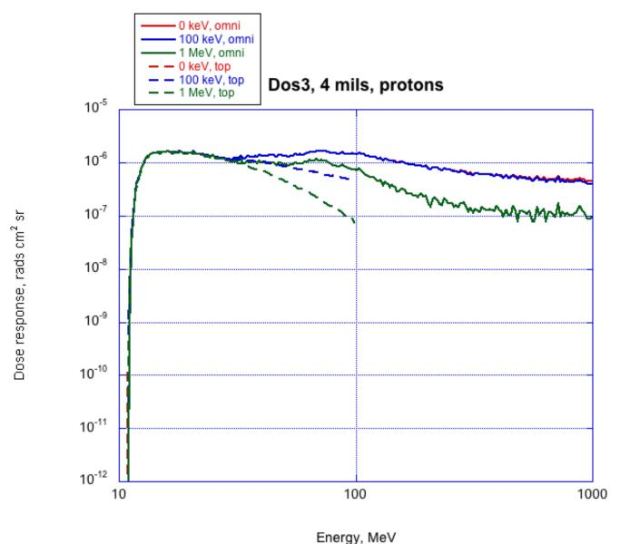
Here is the Dos3 response to protons, with thinned window. I simulated electrons of 10 keV to 10 MeV for both "omni" and "top" illuminations; for protons I simulated 1 MeV to 1 GeV for "omni," but because I realized I had the Dos1/2 foil too thick initially (1.8 mils, rather than 1.8  $\mu$ m!) and 1 MeV was not low enough when I looked at the "omni" results after fixing the thickness, I simulated 100 keV to 100 MeV for "top" illumination.
