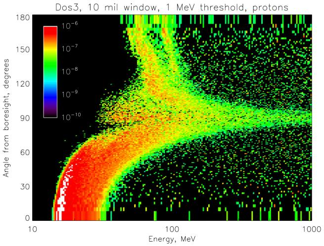
The higher threshold suppresses response at higher energies as dE/dx falls, with a narrow band around 90° surviving as protons at each energy penetrate just enough material that they are nearing the end of their range when they reach the detector.
