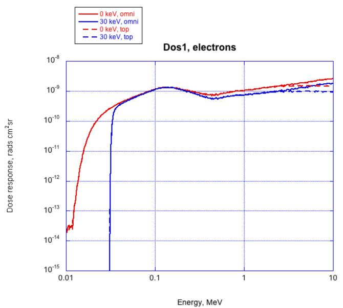
The configuration of the low-energy microdosimeters was a bit more clear to me; both are physically identical, but Dos1 has an electronic threshold of 30 keV and Dos2 has 250 keV. This plot shows the electron response of Dos1, both counting all dose (zero threshold) and after applying the 30-keV threshold.
