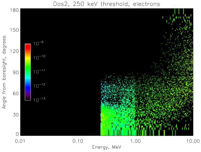
As is seen on slide 10, the high electronic threshold of Dos2 suppresses response to most electron events.
