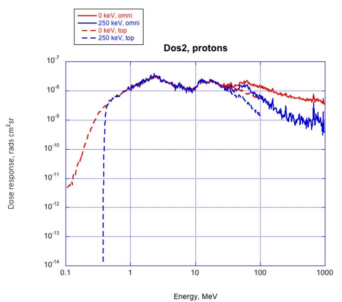
Finally, here is the proton response of Dos2. The 250-keV electronic threshold imposes a sharp turn-on to its response, but most dose is counted from any event until energies reach high enough values that dE/dx drops considerably.
