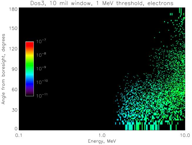
The high threshold, as is clear from slides 5 and 6, greatly suppresses the response. Units on logarithmic colorscale are dose response to particles from the given direction, in rads per (particle per cm<sup>2</sup>) or just rads cm<sup>2</sup> (integrate d $\Omega$  to get the curves in slides 5-12).
