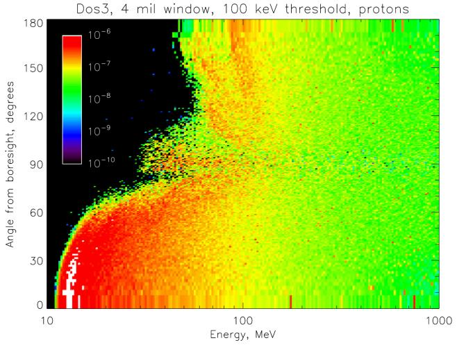
Dos3 proton response with the 100-keV threshold shows a pattern similar to but sharper than that for the electrons on slide 13. This is for the thin window; again, the thick window just shifts the threshold of the main response to the right, leaving the penetrating response the same.
