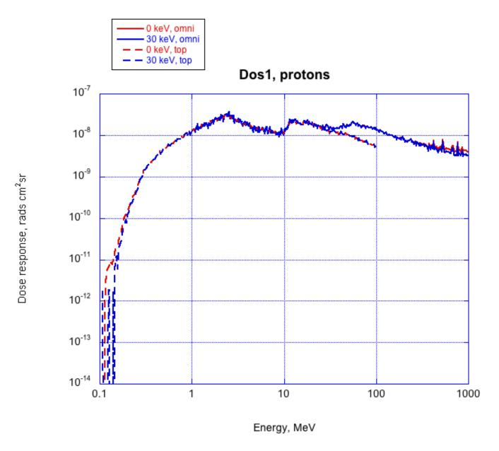
Dos1, with its low threshold, counts nearly all the dose from any proton that can get through the foil or housing to reach its detector.
