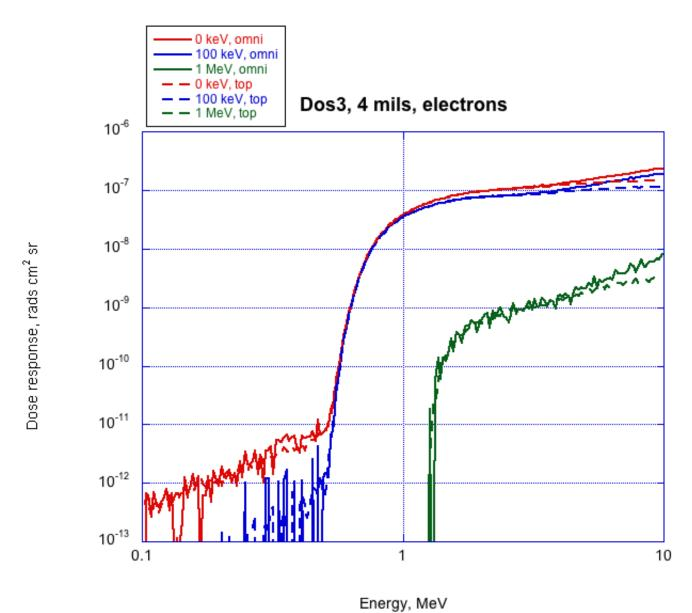
To capture all penetrating response, I illuminated the whole satellite with omnidirectional protons and electrons; I also illuminated just a circle around each microdosimeter on the top to boost statistics at lower (non-penetrating) energies. Since configurations were not completely clear to me, I modeled the Teledyne microdosimeter (Dos3) both with the 10-mil Kovar lid milled to 4 mil above the detector chip, and without; this is with the thinning. 5
