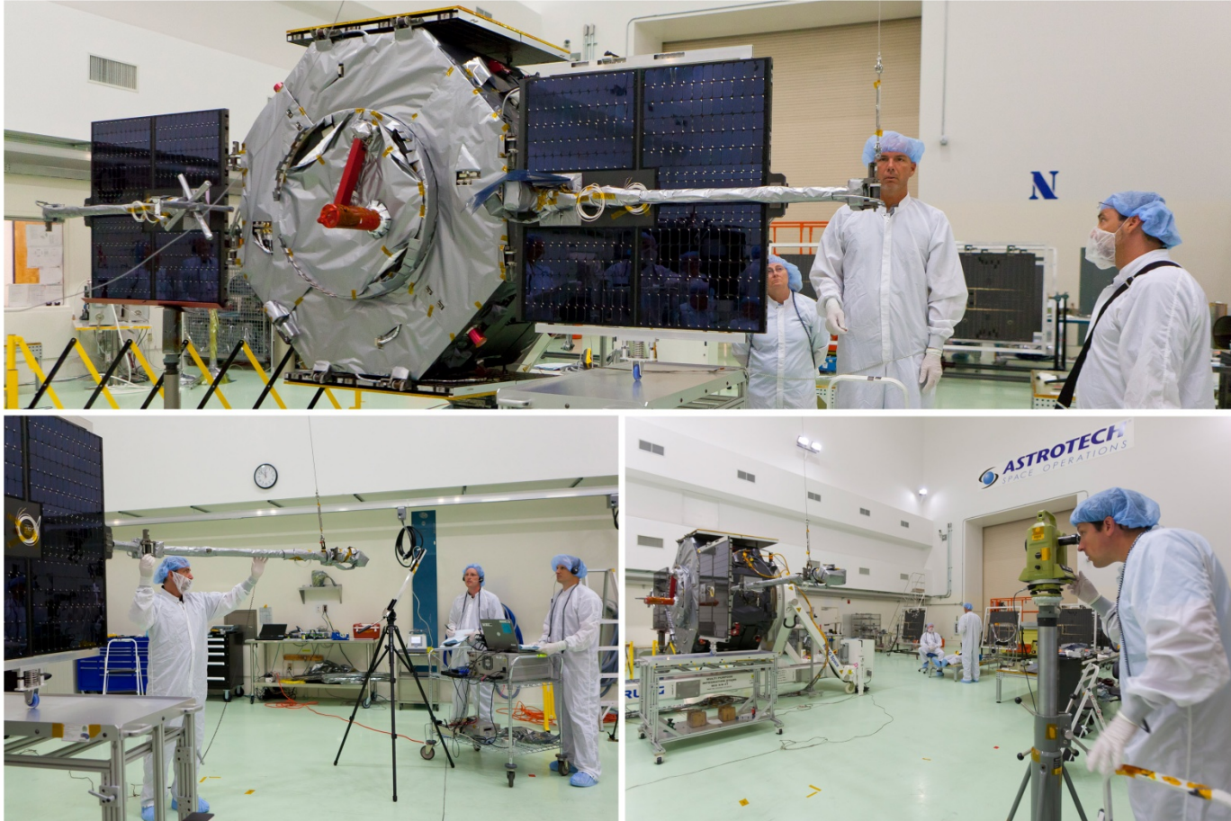
Solar array and boom Deployment testing and final mag boom alignments
