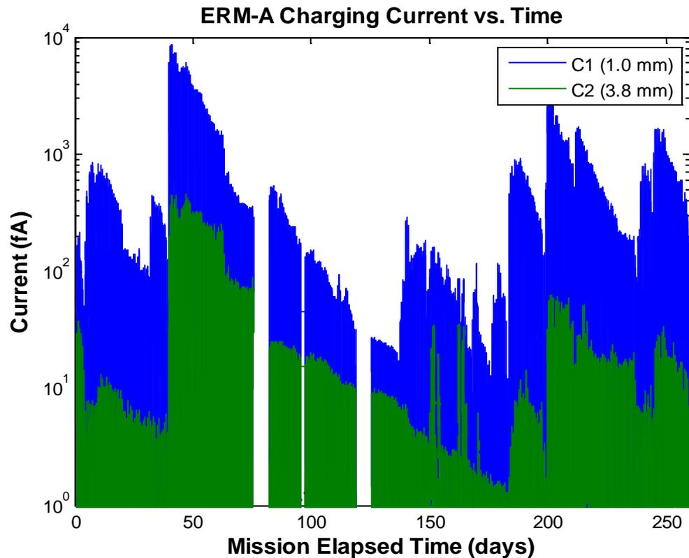
Charge monitor plate currents in femtoamps versus time for electrons  $> 0.7$  MeV (upper blue) and  $> 2$  MeV (lower green). Day 0 is August 30, 2012.
