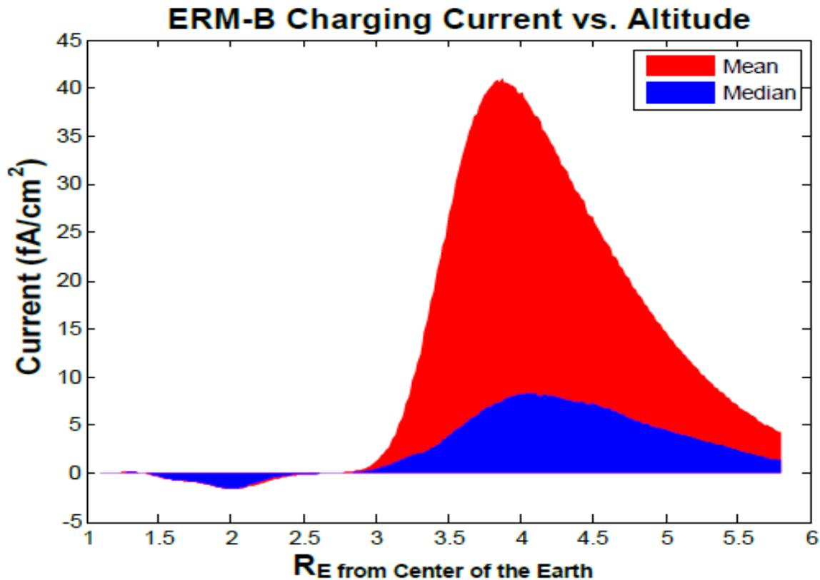
Charging current (electron current as positive) versus orbit altitude for more than 400 orbits below the 1 mm Al cover (electron energy >0.7 MeV; proton energy > 15 MeV). Below ~2.5  $R_E$  protons dominate and the median and mean plots are almost equal due to inner belt stability; above ~3  $R_E$ , electrons dominate and the peak of the mean plot is ~8 times greater than the median plot due to outer belt variability.
