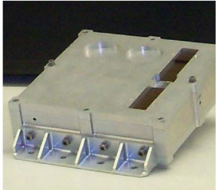
*Left:* Flight ERM with its cover removed showing the locations of the individual RadFET dosimeters and the two charge monitors; the maximum shielded board-mounted RadFET is at the lower right next to and deeper than the RadFET bench; *Right:* view with cover showing variable thickness absorber.
