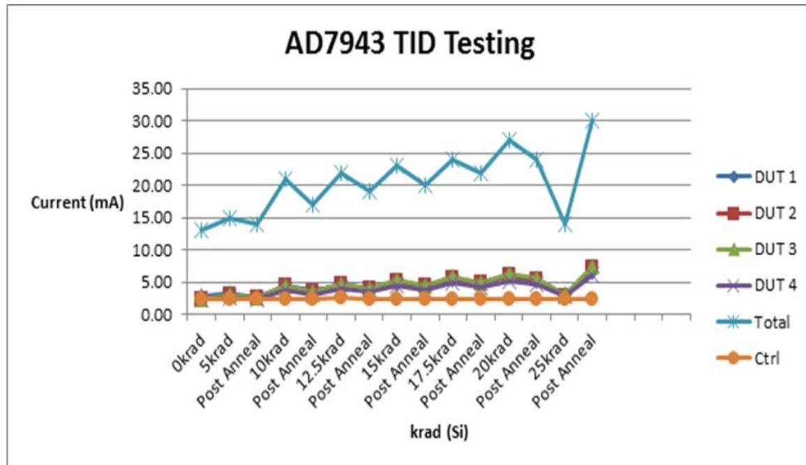
Supply current versus accumulated total dose and anneal cycles for the AD7943 DAC completed in September 2013. The four devices under test survived 20krad; functional behavior became erratic after 25krad.
