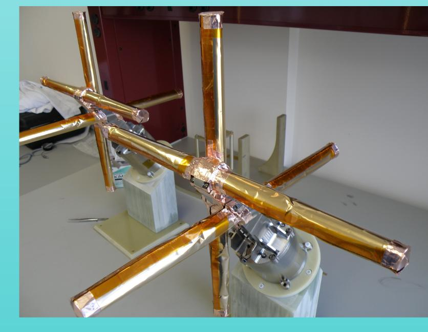
The two triaxial search coil assemblies for Van Allen Probes A and B are shown on pre-launch test fixtures. The search coils consist of 40-cm mu-metal rods and 10,000 turns of fine wire. Radiation tolerant preamps are housed in the cylindrical fixture which doubles as the structure holding the search coils at the end of one of the sensor booms. Performance of this system is excellent, given the superb dynamic range afforded by the 16-b A/D converters used in the 6-channel Wavefrom Receiver
