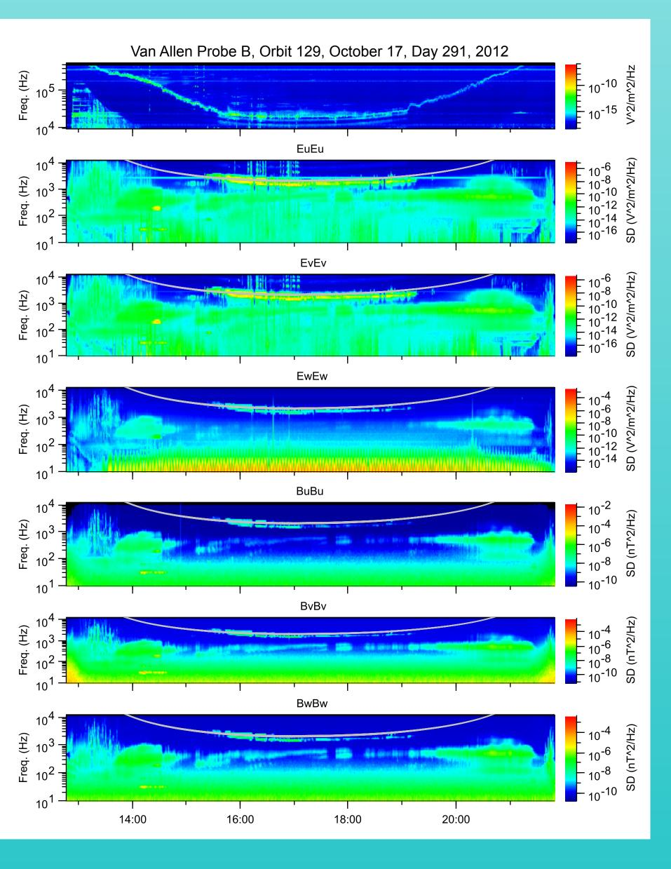
The basic survey output of the EMFI-SIS/Waves instrument is a set of spectral matrices covering the frequency range of 10 Hz to 12 kHz utilizing six channels (3 E and 3 B) and a single-channel spectrum for the HFR frequency range of 10 kHz to 500 kHz. While this spectrogram shows little in the way of amplitude differences between the channels, the spectral matrices capture phase differences between the various wave components and allow later determination of wave propagation parameters.
