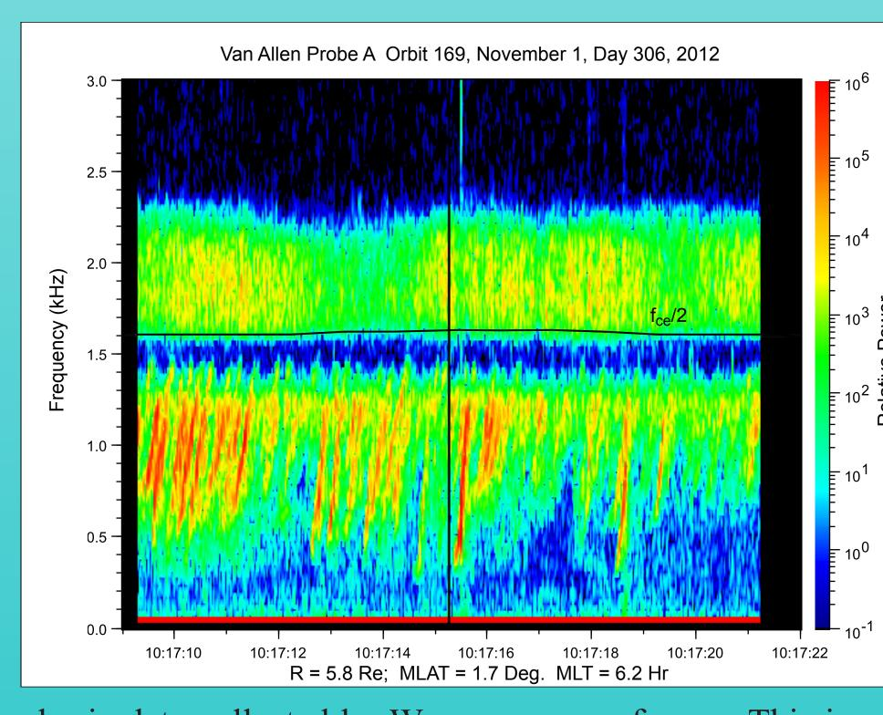
The basic data collected by Waves are waveforms. This is an example of the continuous waveform burst capability, acquired in two 6-second intervals. While all 6 components are captured, this panel only shows the spectrum for the  $B_u$  component. An onboard algorithm selects such captures based on the amplitudes in the chorus bands above and below  $f_{ce}$ . The EM-quiet spacecraft and 16-b dynamic range make for an excellent data set.
