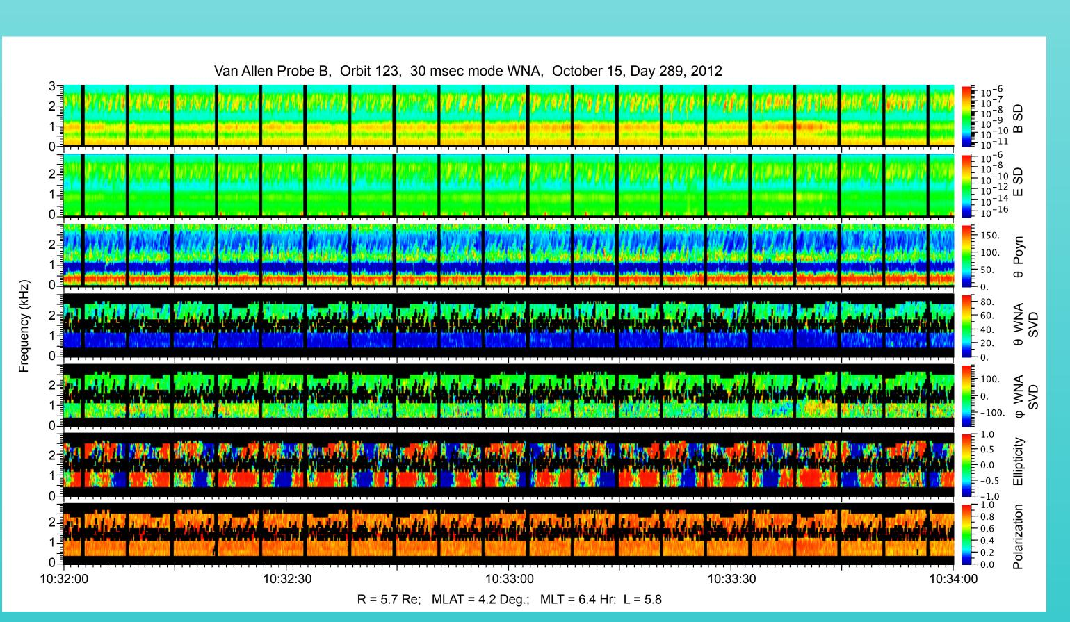
A basic capability of the Waves multi-component waveform measurements is the determination of wave propagation characteristics such as wave-normal angle, Poynting flux, polarization, etc. These parameters -- magnetic and electric spectral density, polar angle of the Poynting flux, wave-normal angles, ellipticity, and polarization were all computed on-board at 30 msec intervals. As is now expected, the chorus near 2 kHz propagates away from the equator.
