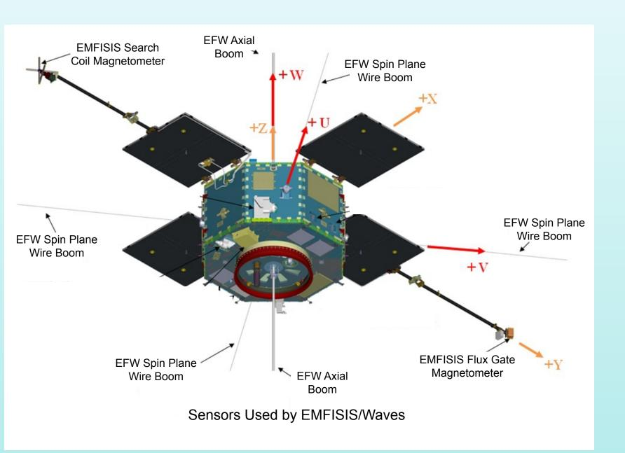
The EMFISIS/Waves instrument on the twin Van Allen Probes utilize a complete array of plasma wave sensors. Three orthogonal components of the wave magnetic field are obtained from a triaxial search coil magnetometer on a 3-m boom. Three orthogonal electric field components are obtained from the EFW (Electric Fields and Waves) sensors including 2 spin plane booms 100 m tip-to-tip and an axial boom approximately 13.4 m, tip-to-tip.
